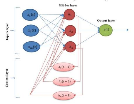
Fig. 2. Architecture of Elman recurrent neural network
